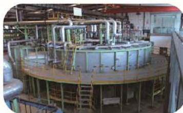
Rotary hearth furnace clean smelting technology to ferrous and non-ferrous metal ores
