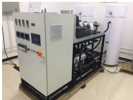
Ejector expansion CO 2 heat pump coupled with thermal storages
