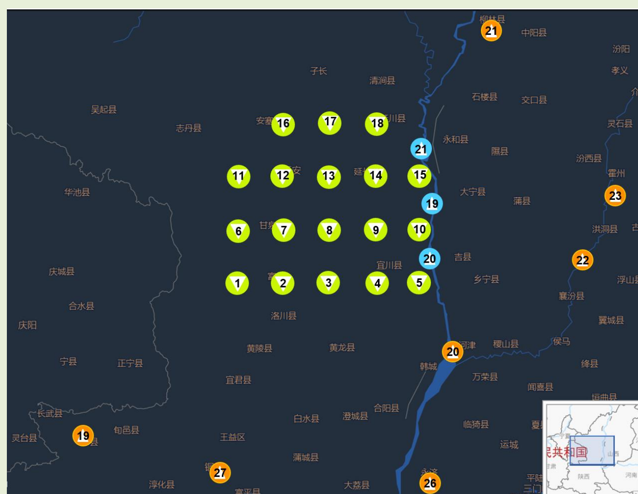
Fig. 1. Schematic of potential shale gas sources (green), water acquisition sites (blue) and CO 2 sources (orange) in Ordos Basin.
