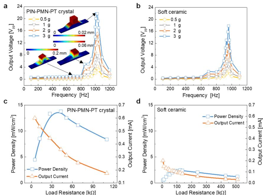
**Fig. 3** Energy harvesting performance of BSPEH. (a)(b) Output voltage; (c)(d) output power density and current.
