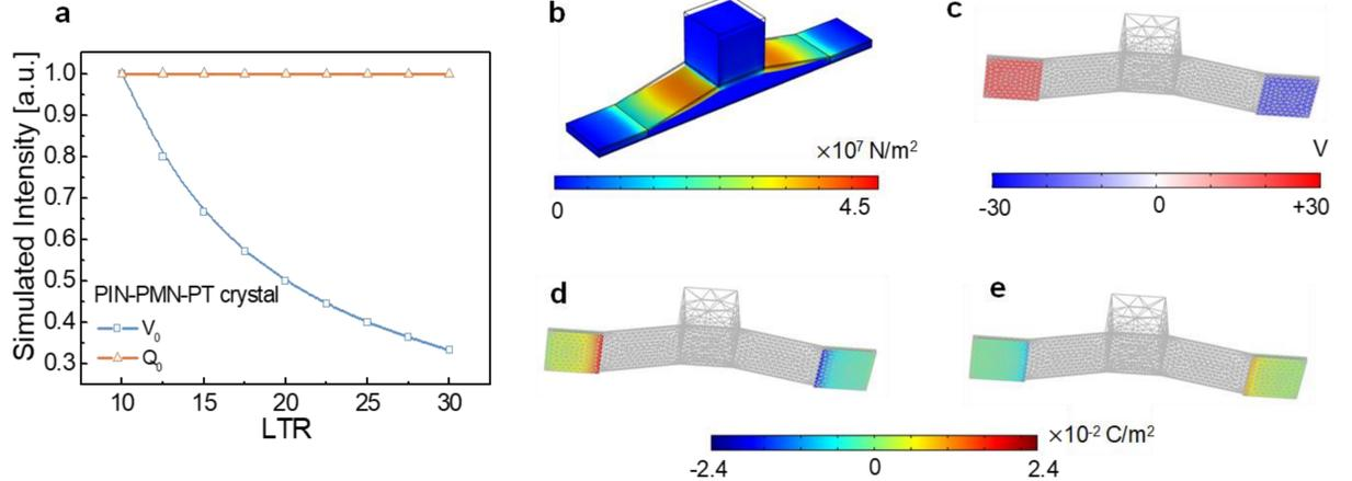
**Fig. 2** Output voltage and charge density of BSPEH by FEM simulation. (a) Open circuit output voltage ( $V_0$ ) and short circuit charge density ( $Q_0$ ) with different length to thickness ratio (LTR). (b) Stress distribution and (c) output voltage at resonance frequency; and output charge density in short circuit for (d) PIN-PMN-PT crystal and (e) soft piezoelectric ceramic.
