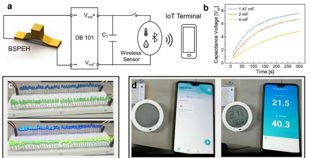
**Fig. 4** Practical applications. (a) Circuit diagram for powering wireless sensors in IoT system. (b) Charging behaviour for different capacitance. (c) 200 LEDs are lit up. (d) Wireless sensing powered by the BSPEH.
