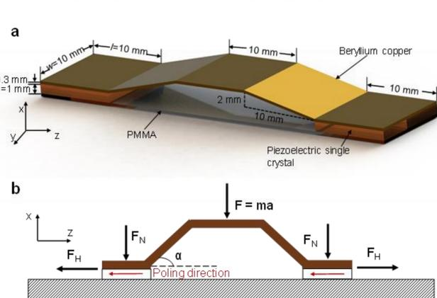
**Fig. 1** Working principle of the BSPEH. (a) Schematic of the energy harvester; (b) Mechanical analysis of the structure.
